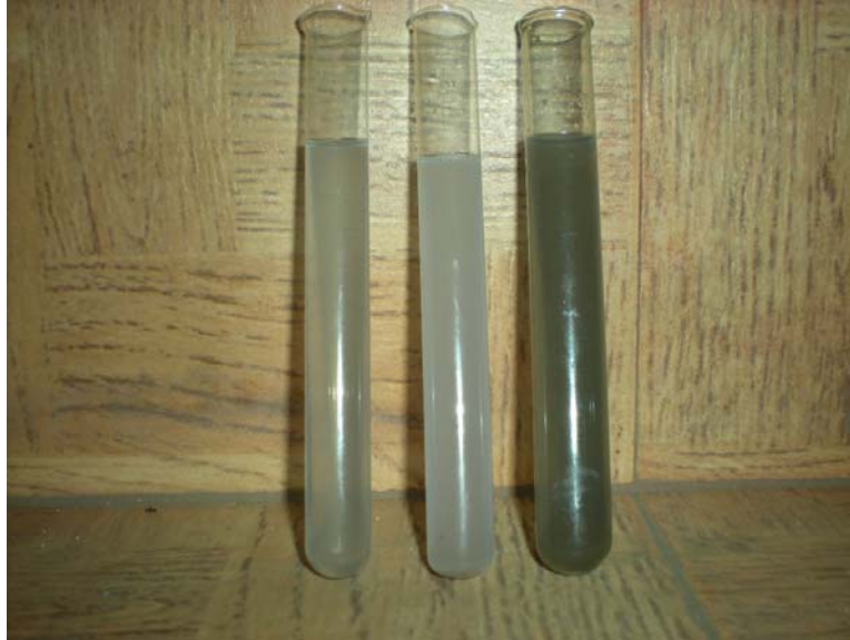
Fig 4.17 Photographs of Al-H 2 O (Left), Cu-H 2 O (Middle), and Al-Cu-H 2 O (Right) suspensions in presence of oleic acid surfactant.
