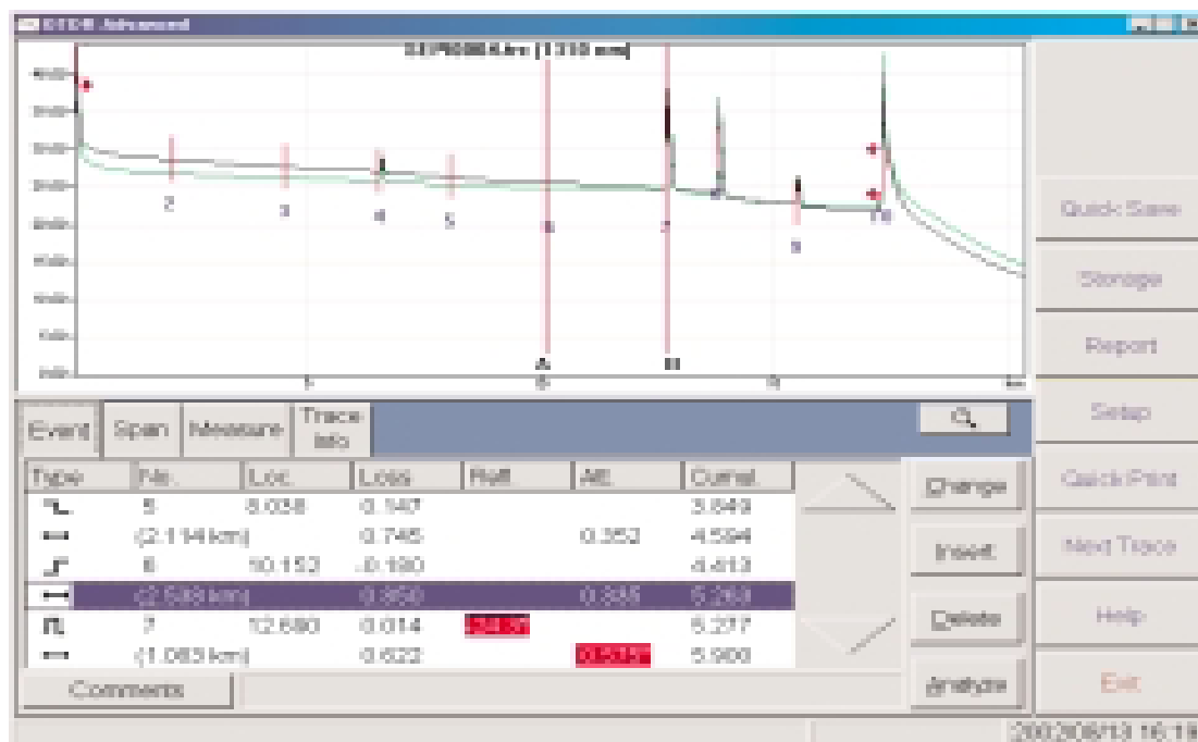
Fig. 1.1: A typical OTDR trace screen. [45]
