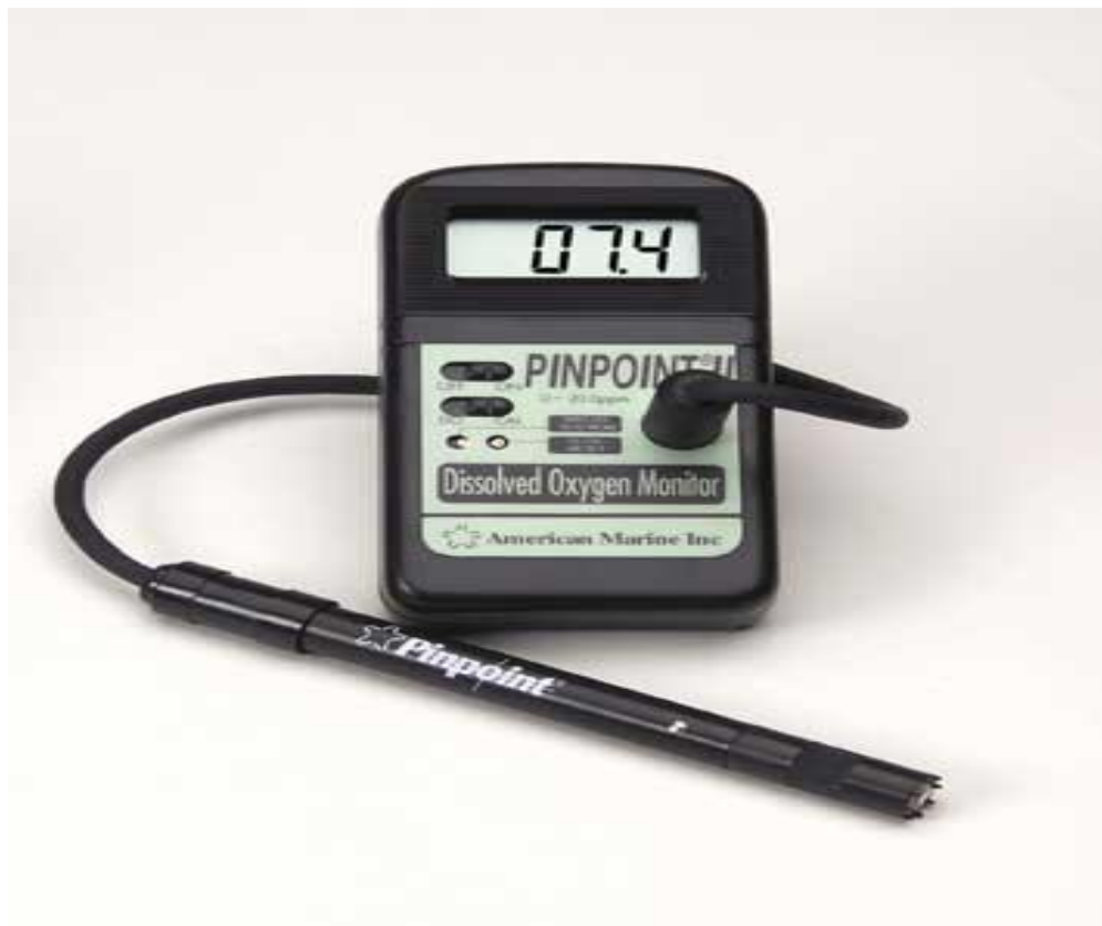
Fig 6.4: Device to measure dissolved oxygen
