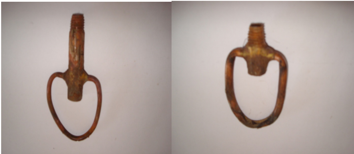
Fig. 3.12 U-Shaped tubular electrode of dia 4mm & 6 mm for machining step 1 & 3
