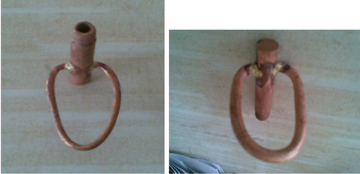
Fig. 3.11 U-Shaped tubular electrode of dia 4mm & 6 mm for machining step 2
