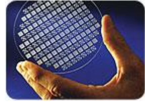
Square cavities, round through holes and crossing beams in a 4-in. borosilicate wafer.
