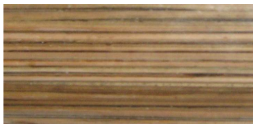
Figure 3. Specimen of coconut fiber reinforced epoxy composites
