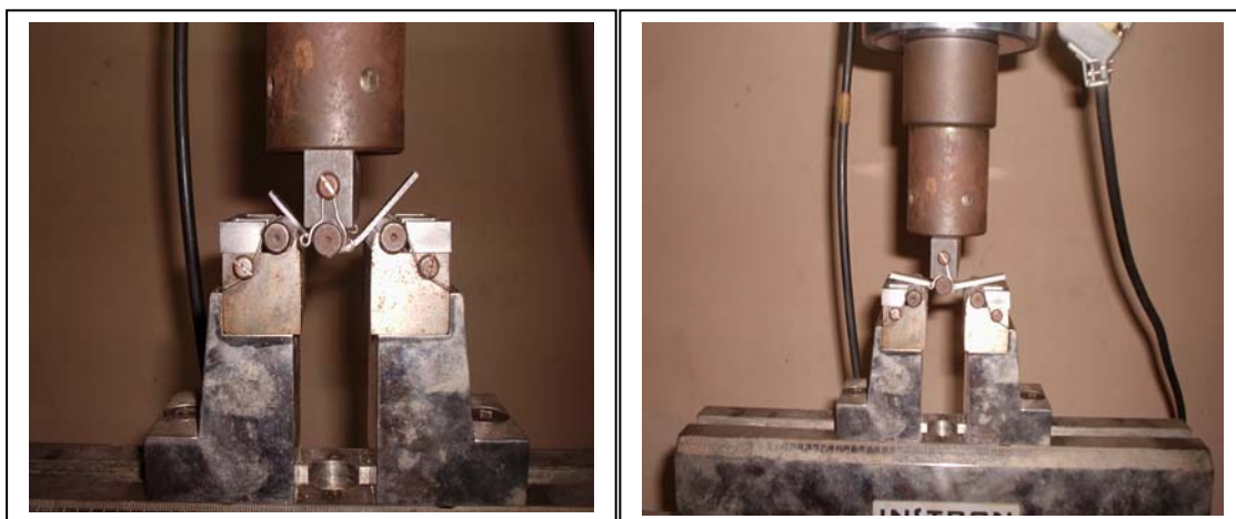
Fig 3.3(a) Photograph of the machine (Instron 1195) for 3 point bend test
