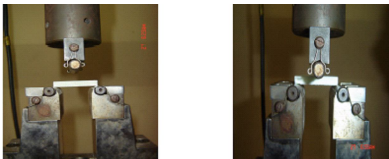
Fig 4.4 Short Beam Shear test set up, loading of the sample
