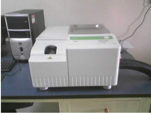
Fig.4.1. (a) Mettler-Toledo 821 with intra cooler for DSC measurements and (b) reference-sample chamber.
