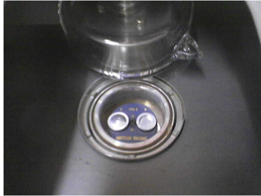
Fig.4.1. (a) Mettler-Toledo 821 with intra cooler for DSC measurements and (b) reference-sample chamber.
