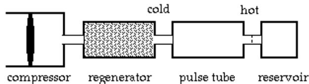
**Fig: 1.2 Orifice Pulse Tube**
