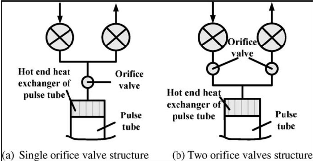
Fig: 4.1 Orifice valve structures
