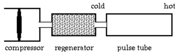
**Fig : 1.1 Basic Pulse Tube Refrigerator**
