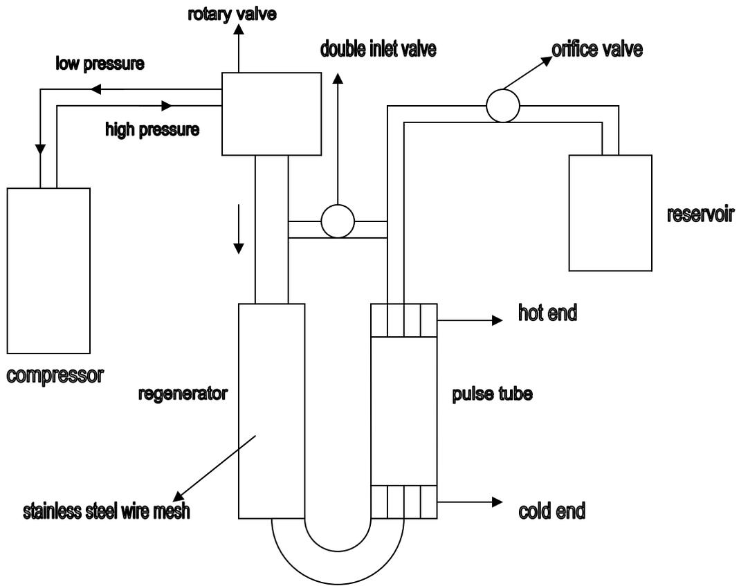
**Fig: 6.1 Schematic diagram of pulse tube refrigerator**
