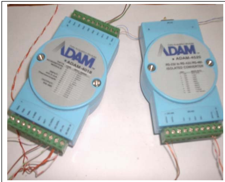
Figure 5.7 Photograph of data acquisition system (ADAM module 4018 and converter 4520).
