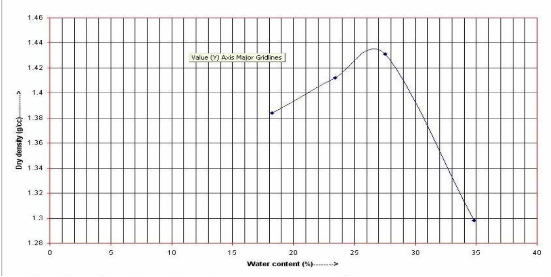
Fig-9: Proctor compaction Test with swelling soil+30% fly-ash
