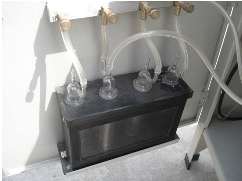
Figure-5.3: Gaseous sampling arrangement for Respirable dust sampler
