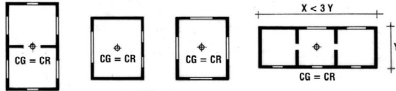
Fig 1.5 Proper distribution of Walls and openings
