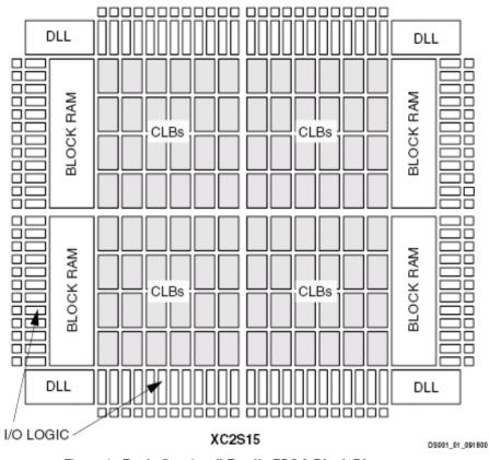
Figure 1: Basic Spartan-II Family FPGA Block Diagram
