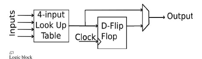
There is only one output, which can be either the registered or the unregistered LUT output. The logic block has four inputs for the LUT and a clock input. Since clock signals (and often other high-<u>fanout</u> signals) are normally routed via special-purpose dedicated routing networks in commercial FPGAs, they and other signals are separately managed.
