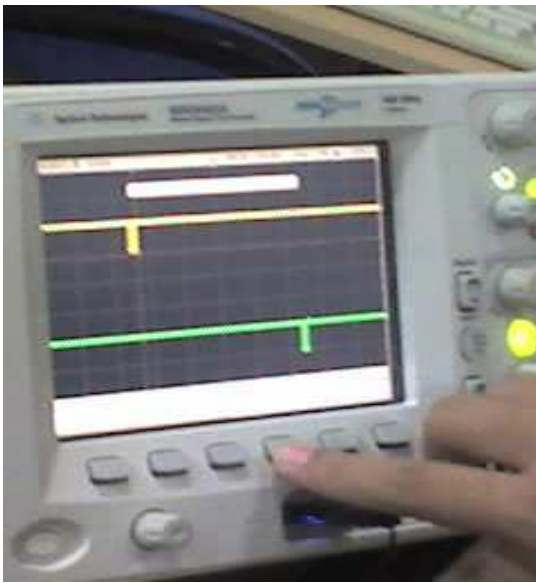
Figure 6.3. Tx and Rx lines with ECHO being ON.
