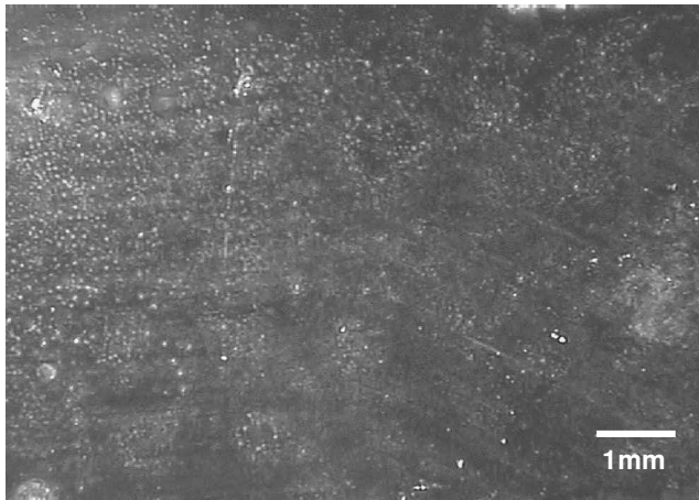
Fig. 1 Typical surface morphology of the HPDL-fired enamel glaze on the mild steel (2 kW/cm 2 power density, 480 mm/min traverse speed)
