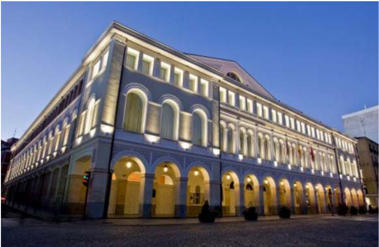
Image 100 302 . Rutas ríos de luz. Valladolid, España. The full facing facades are not illuminated, but only certain elements are highlighted.
