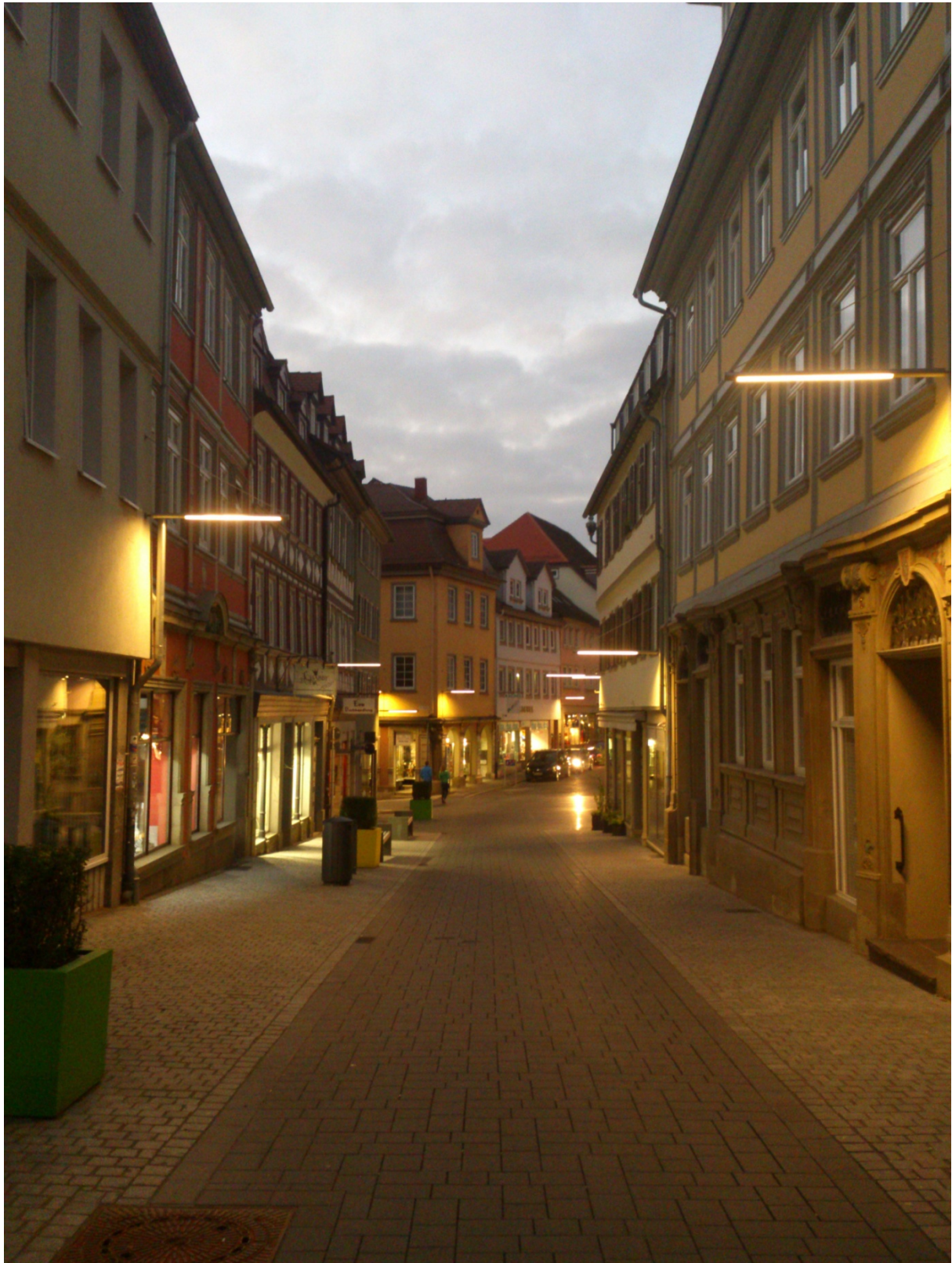
Image 102 305 . Streetlights of Marktsraße in Schwäbisch Hall, Germany, 2013. The luminaires are recessed directly on the walls and their light projection is enough to see at night. The color of the light is amber.
