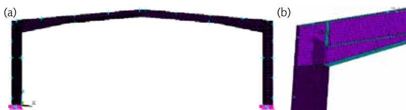
Figure 2 — a) Shell model (Ansys), b) Details of the shell model
