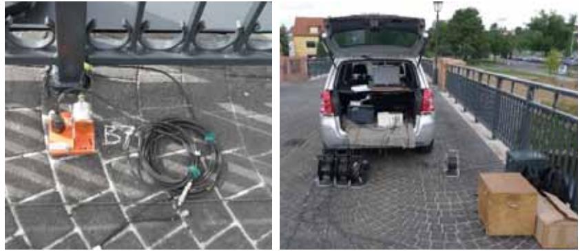
Figure 4 — Accelerometer and measurement equipment
