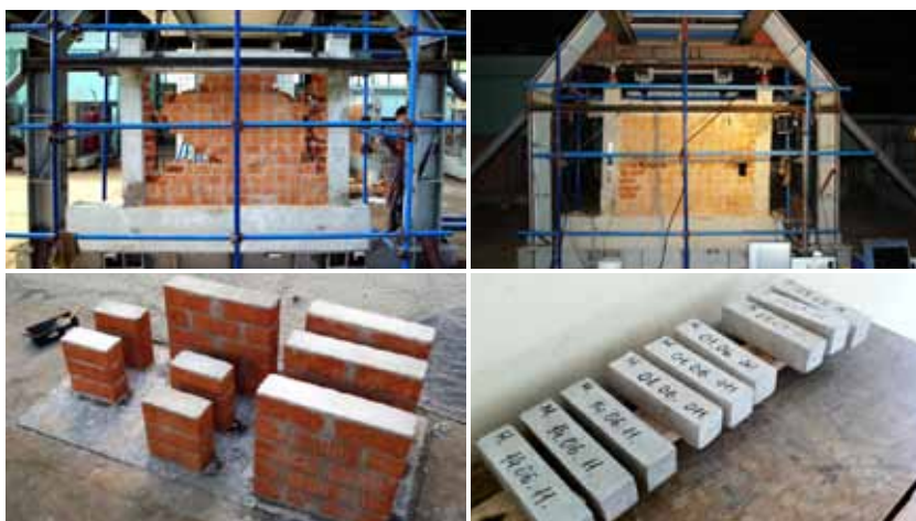
Figure 7 – View of the experiment in progress and associated samples of masonry and mortar
