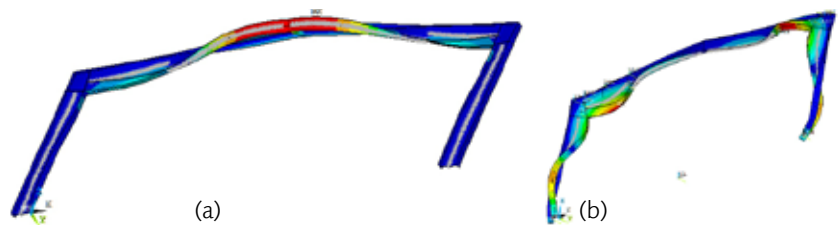
Figure 8 — (a) Lateral-torsional buckling B, (b) Lateral-torsional buckling C
