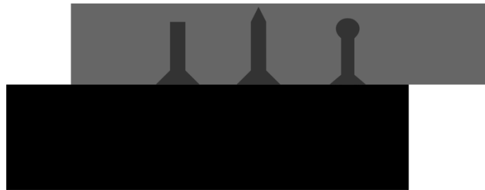
Figure 1: Schematic representation of differently shaped pins. The black bulk represents the base material and the light gray area is the attached part.
