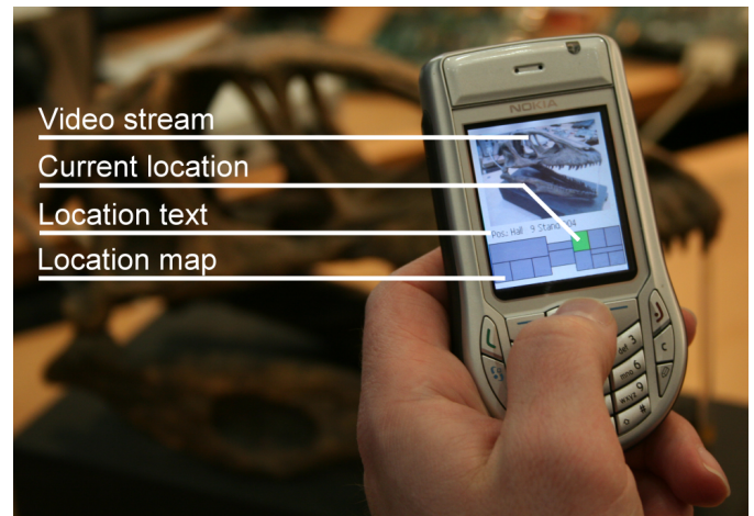
Fig. 8 Object recognition with PhoneGuide: Elements of the user interface are annotated.
