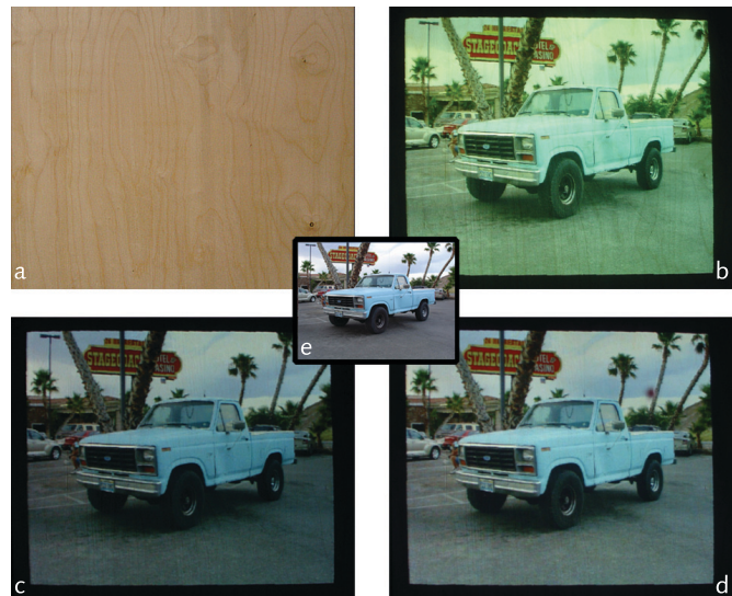
Fig. 8. Projection onto a wooden surface, without (b), with manually adjusted (c) and with adaptive radiometric compensation (d).
