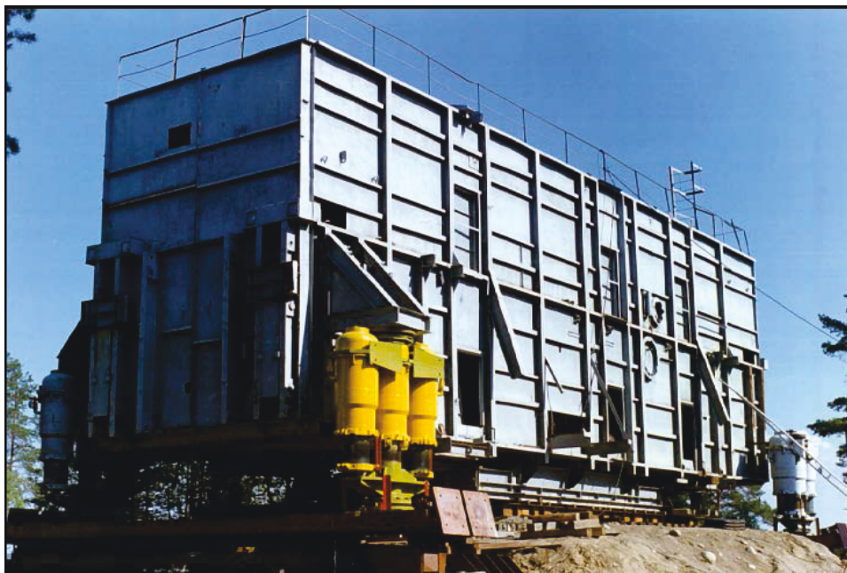
Figure 2.2. Shock-proof object with shock-absorber units.
