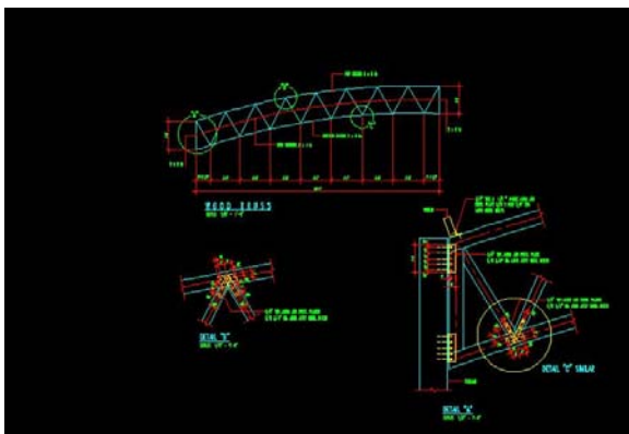
Figure 1a: Boathouse truss and truss connections detail.
