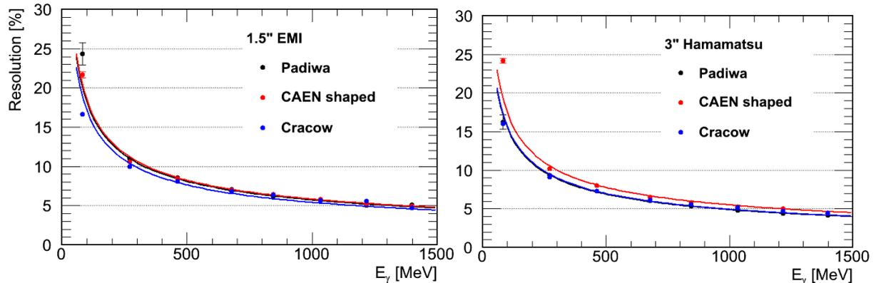
**Figure 1.** Relative energy resolution measured with the standard CAEN ADC and novel front-end boards “Cracow” and PaDiWa Amps. Data are measured using the module with 1.5” photomultiplier (left) and 3” photomultiplier (right).
