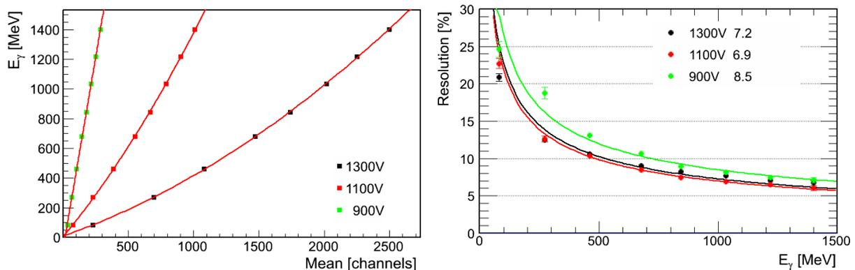
**Figure 2.** The (non)linear response of 1” Hamamatsu R8619 photomultiplier as a function of high voltage (left). Relative energy resolution of ECAL module equipped with 1” Hamamatsu R8619 photomultiplier as a function of high voltage (right). Numbers behind the names stand for resolution with 1 GeV photons.
