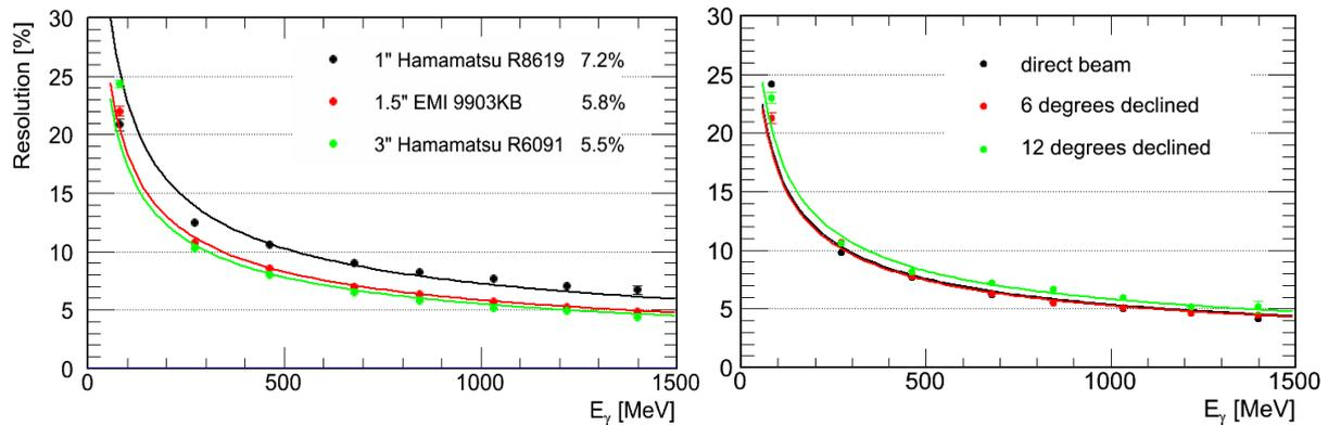
**Figure 3.** Comparison of relative energy resolution for modules with PMTs of different size (left). Relative energy resolution of the ECAL module equipped with 3" PMT with respect to the various declination of the incident photon (combination of measurements with different angle) (right).
