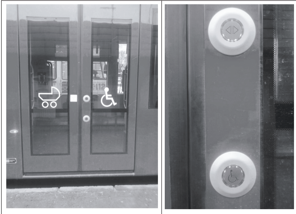
Photo 5. Additional buttons for people with disabilities to open doors in public transport (Marcin Popiel)
