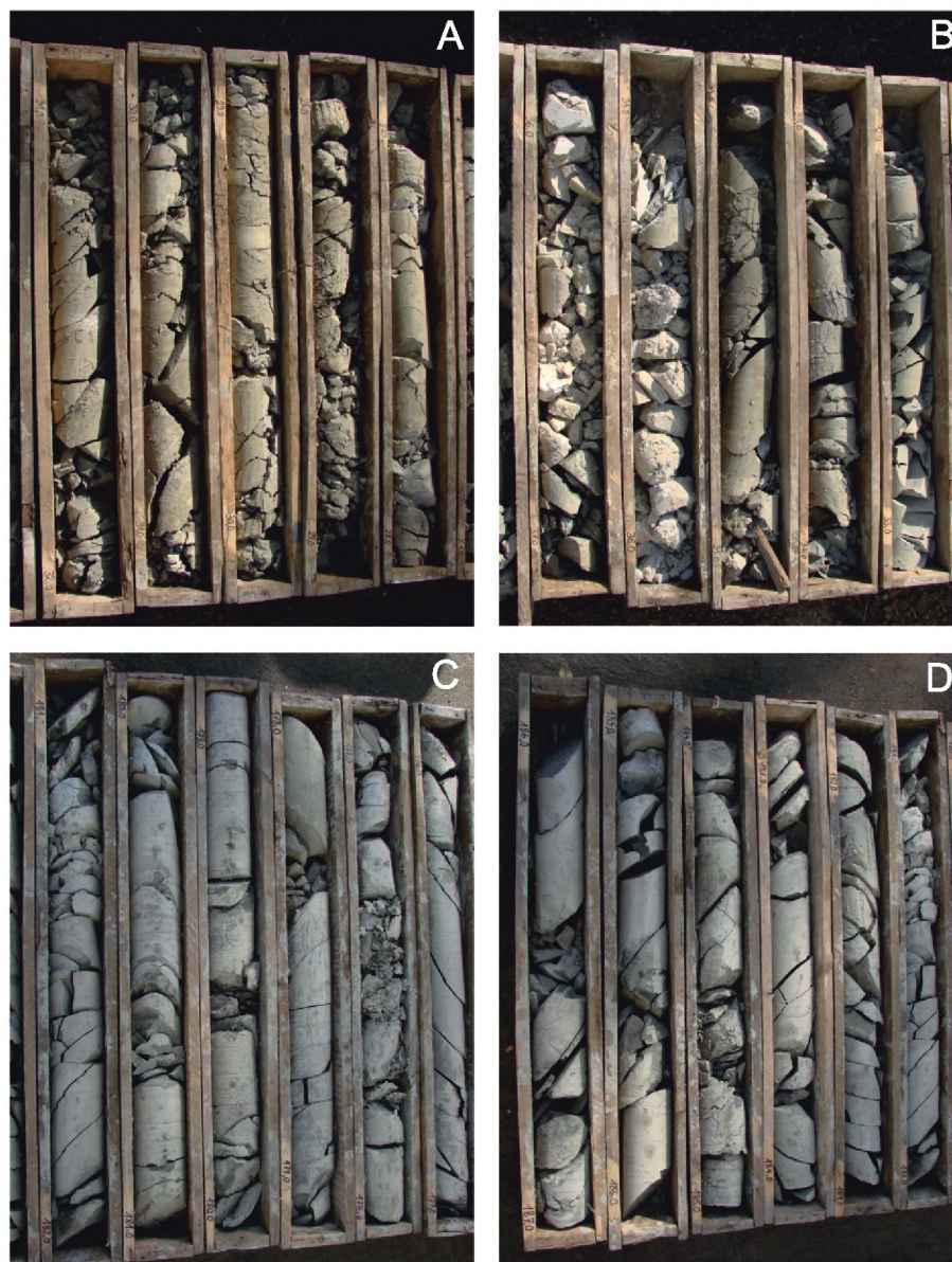
Fig. 6. Pilzno P-7 borehole – core photographs showing steep inclination of the Sarmatian foredeep infill within the deformed Zgólskie Unit
