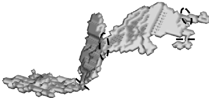
Figure III-11. Example of hole object with multiple 1-voxel thin connexions, also known as isthmuses (dashed lines). Encircled connexions present a larger width. Figure published in [Babout and Janaszewski 2009]
