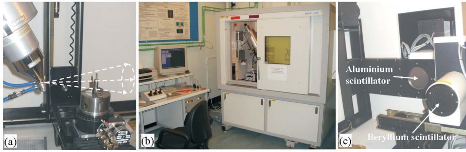
Figure I-3. X-tek HMX X-ray tomography system. (a) lateral view of X-ray gun and rotation stage showing schematic representation of X-ray cone beam (b) general view of the hutch (c) detectors (aluminium / beryllium scintillators coupled with 1024x1024 CCD camera). Pictures taken by the author with consent of the equipment's owner (i.e. SDC-MMSC; head of Unit: Prof. P.J. Withers)
