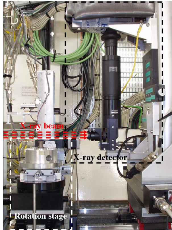
Figure I-2. Lateral view of the X-ray tomography setup developed at ID19 beamline (ESRF). Picture taken by the author with consent of the equipment's owner (i.e. ID19 beamline; head of Unit: dr J. Baruchel)
