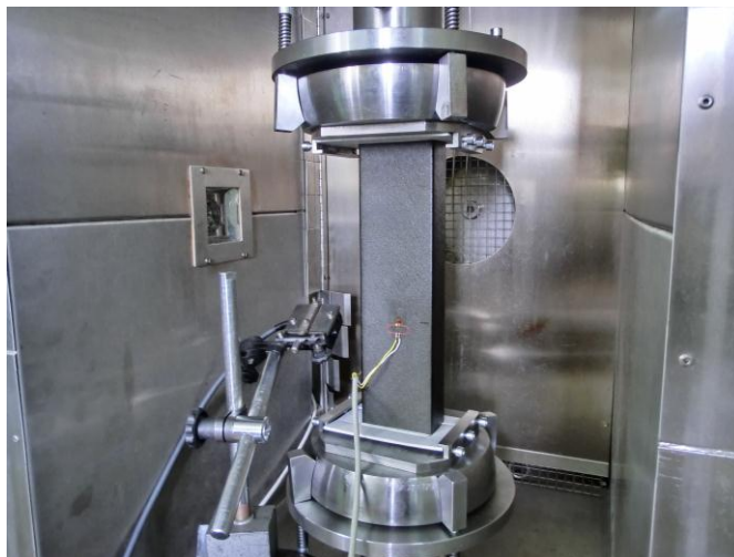
Fig. 3. Stand test with self-aligning grips for compressive loading of composite columns
