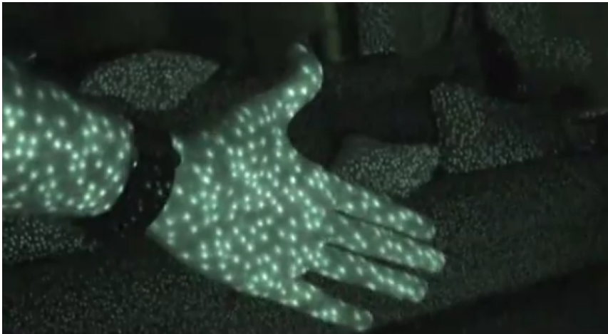
Figure 6. Marking the room with infrared beams by Microsoft Kinect [7]
