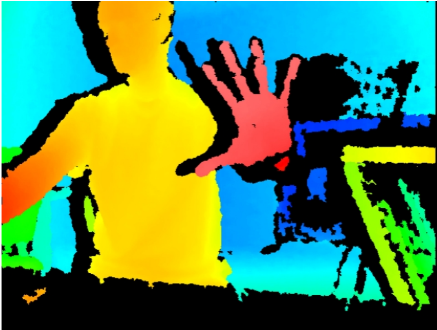
Figure 7. Sample depth map created by Microsoft Kinect [7]
