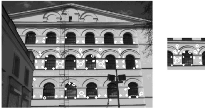
Figure 10. Comparison of the template training image (right) with the tested image of the White Factory in Lodz. The white points indicate elements recognized in both figures.
