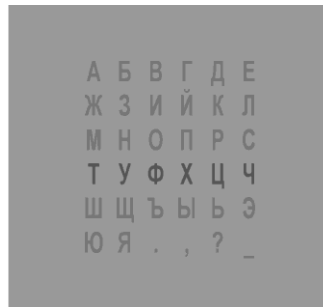
Figure 1. The method of organization of brain-computer interface called "request-response"
