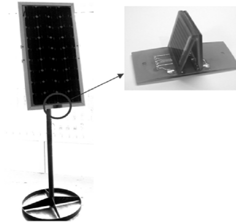
Fig. 7. The experimental model of the solar tracking system
