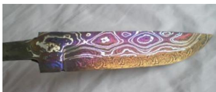
Pic. 1- Knife blade decorated using the method of high temperature oxidation.
