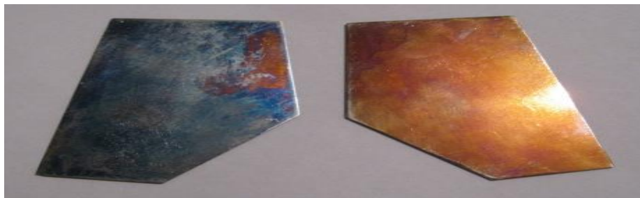
Pic.4 Defects of oxidation
