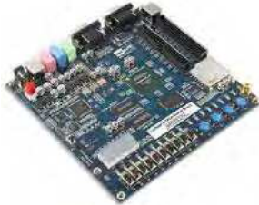
Fig. 2. Exterior of the Cyclone II Starter Development Board
