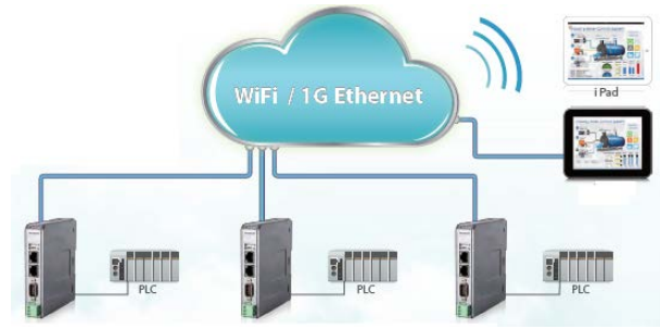
Figure 3. cloud based HMI architecture
