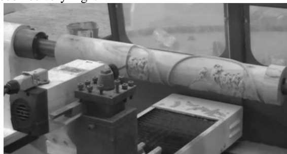
Figure 2. Production of balusters on a lathe CNC
