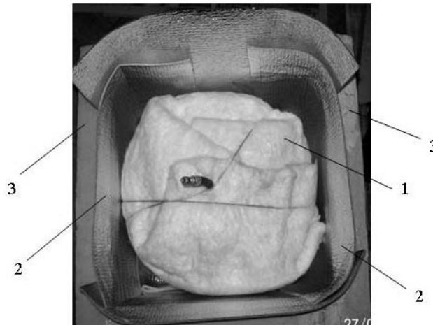
Figure 5. Thermoinsulated hydraulic accumulator: 1 - basalt fiber; 2 - penofol; 3 - extruded polystyrene foam.
