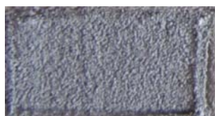
Figure 1. Appearance of the sintered surface PA-4 (x2), Sintering modes V=1000 mm/min, t=26 °C, S=0.2 mm, P=10 W.
