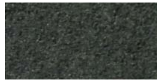
Figure 22. Appearance of sintered surface DSK-F75 (x2), sintering modes P=10 W, t=26 °C, V=300 mm/min S=0.15 mm.
