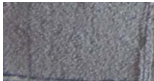
Figure 17. Appearance of sintered surface PA-4 (x2), sintering modes P=10 W, t=26 °C, V=1000 mm/min, S=0.1 mm.
