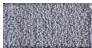
Figure 7. Appearance of the sintered surface PA-4 (x2), sintering modes P=20 W, t=26 °C, S=0.2 mm, V=1000 mm/min.
