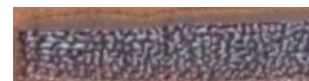
Figure 12. Appearance of the sintered surface PMS-1 (x2), sintering modes V=200 mm/min и P=30 W, t=200 °C, S=0.1 mm, V=3000 mm/min.
