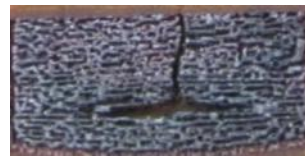
Figure 4. Appearance of the sintered surface of PMS-1 (x2), Sintering modes V=200 mm/min, t=200 °C, S=0.3 mm, P=30 W.
