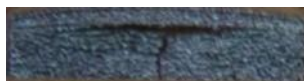
Figure 11. Appearance of the sintered surface PMS-1 (x2), sintering modes V=200 mm/min и P=30 W, t=200 °C, S=0.1 mm, V=200 mm/min.
