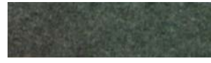
Figure 16. Appearance of sintered surface DSK-F75 (x2), sintering modes P=10 W, t=26 °C, S=0.1 mm, V=300 mm/min.
