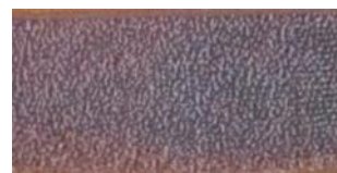
Figure 14. Appearance of sintered surface PMS-1 (x2), sintering modes P=22 W, t=114 °C, S=0.2 mm, V=3000 mm/min.
