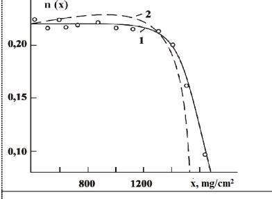
**Figure 3.** Dependence of the concentration on the depth of molybdenum irradiated by protons with energy of 30 MeV; 1 – experiment; 2 – calculation by CP-method at T = 100 keV
