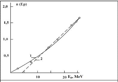
**Figure 4.** Power dependence of complete concentration of the defects created by protons along all the track in Mo 1 – experiment; 2 – calculation by CP-method at T = 100 keV
