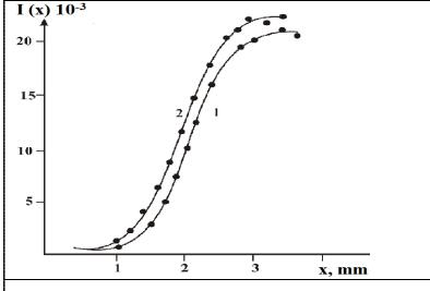
**Figure 2.** Dependence of annihilation photons intensity on the displacement of annealed (1) and the defect (2) samples
