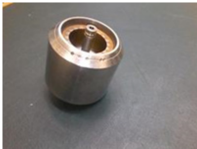
Rotor of a two stator gyromotor
