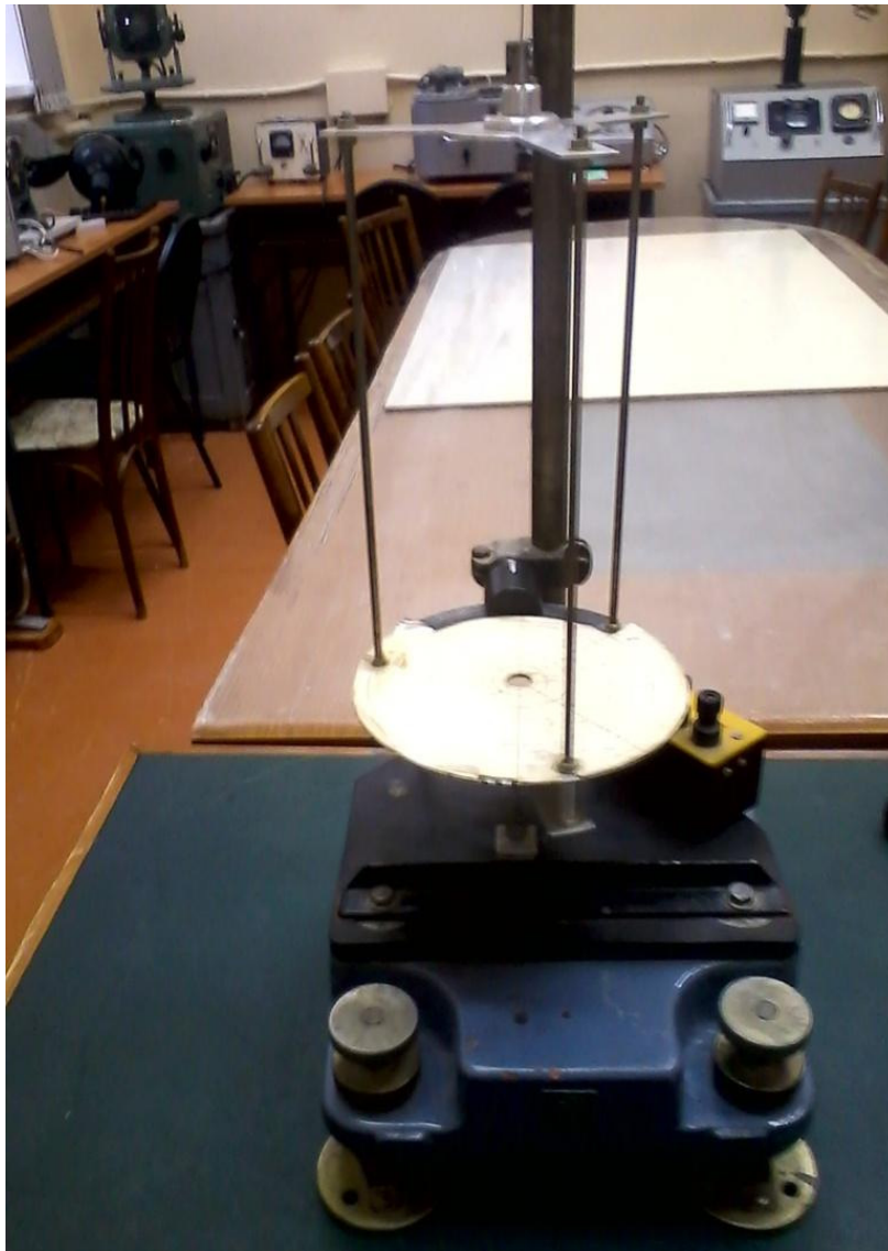
Fig. 1. Installation for definition of the moments of inertia
