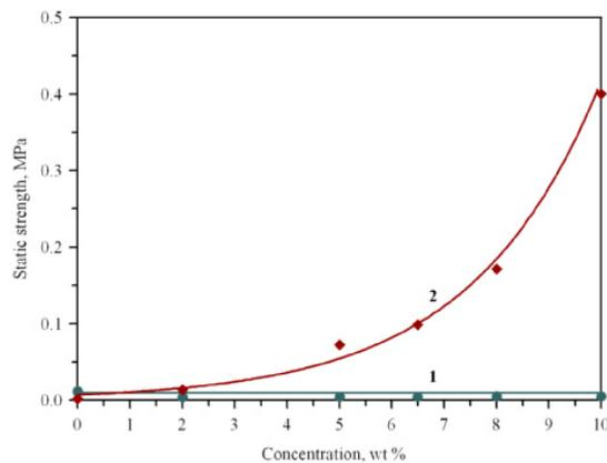
Fig. 5. Influence of liquid sodium glass concentration on static strength of freshly prepared (1) and dried (2) granules
