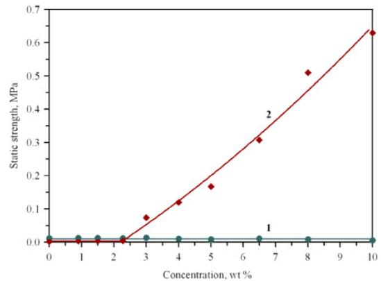
Fig. 4. Influence of glyoxal concentration on static strength of freshly prepared (1) and dried (2) granules
