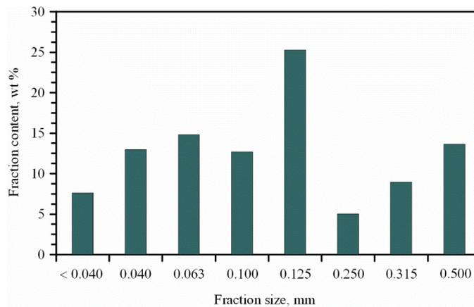
Fig. 1. Particle size distribution of ash and slag material
