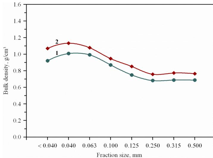
Fig. 2. Dependence of loose bulk density (1) and packed bulk density (2) of ash and slag material of Seversk CHPP on the particle size
