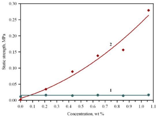
Fig. 3. Influence of polyvinyl alcohol concentration on static strength of freshly prepared (1) and dried (2) granules
