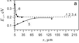
**Figure 1.** The depth distribution of activation energy *Ea* for A (a) and B (b) samples before annealing (curves 1) and after high vacuum annealing (curves 2), annealing in nitrogen (curves 3), annealing in oxygen (curves 4), annealing in nitrogen plasma (curves 5), annealing in oxygen plasma (curves 6).
