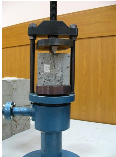
Figure 1. Photograph of the loading system.
