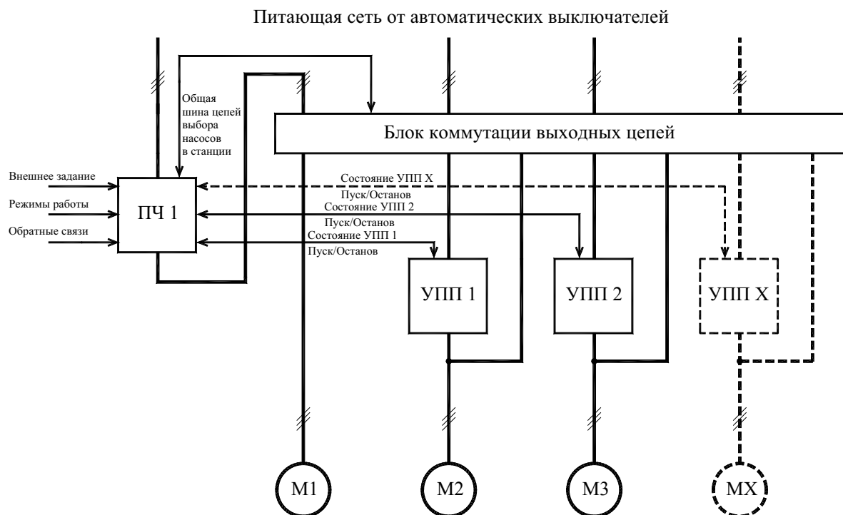
Fig. 3. Functional diagram of the control system of pump station with one frequency converter and smooth start devices: UPP 1, UPP 2, UPP X – thyristor devices of smooth start
