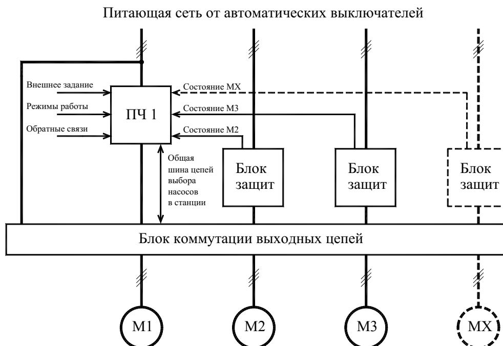
Fig. 2. Functional diagram of the control system of pump station with one frequency converter: M1, M2, M3, MX are the induction motors of the pumps in the station; ПЧ 1 is the frequency converter
