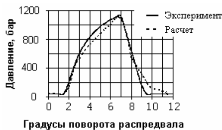
Fig. 3. Characteristics of injection pressure
