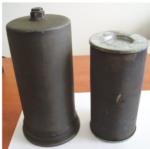
Fig. 10. Ready-assembled oil filter (on the left) and filter element
