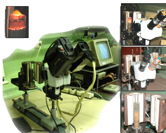
Fig. 1. Experimental complex of micro-pyrometric and optical devices for studying processes of formation of thermal structures in the wave of SH-synthesis
