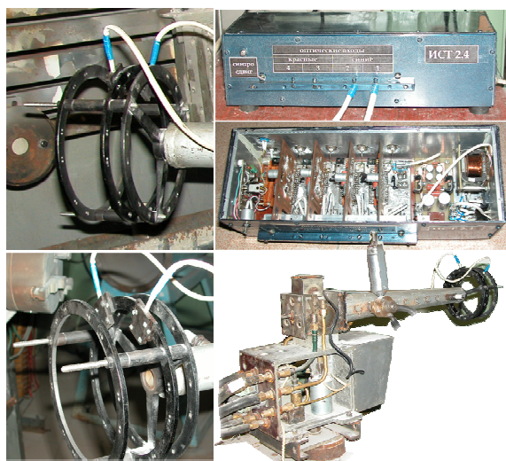
Fig. 3. Experimental stand of studying pulse gas-dispersed flows
