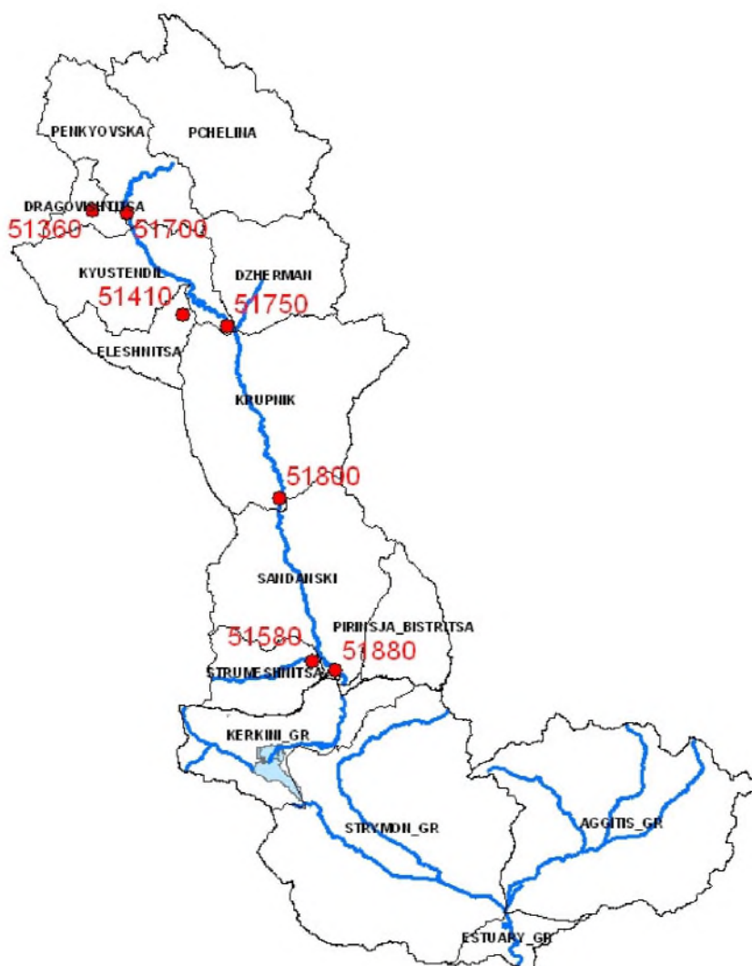
Fig. 2.4. Location of discharge stations used for calibration of Rainfall-Runoff model
