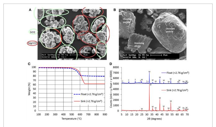
FIGURE 2 | (A) SEM-EDX characterization of reaction products (carbonate- and silica-rich particles indicated); (B) SEM-EDX characterization of reaction products (residual olivine and chromite-rich particles indicated); (C) TGA analysis of dense liquid-separated reaction products; (D) XRD analysis of dense liquid-separated reaction products; (C, clinochlore; F, forsterite; M, magnesite).
