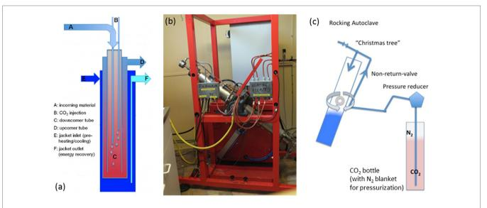
FIGURE 1 | (A) Conceptual layout of "CO<sub>2</sub> Energy Reactor<sup>TM</sup>" (not to scale) (Santos et al., 2013, licensed under CC BY-NC-ND 3.0); (B) lab-scale "rocking autoclave" at ~45° rotation; (C) schematic of "rocking autoclave."
